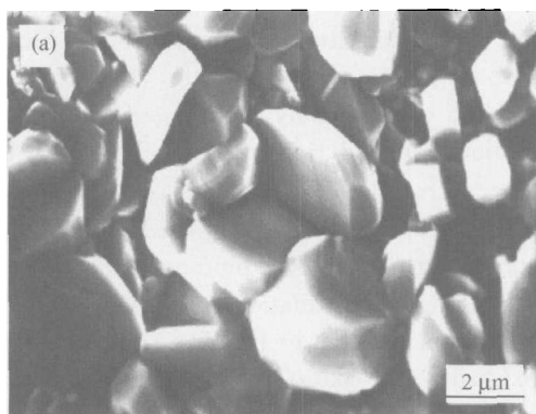
Fig. 3. SEM morphologies of oxide films formed on (a) Co-40Cr and (b) Y-implanted Co-40Cr after 24 h isothermal oxidation.
